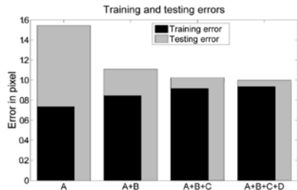
Fig. 2. Training with speaker A, A and B, and so on, and always test by speaker E which is not involved in the training set
